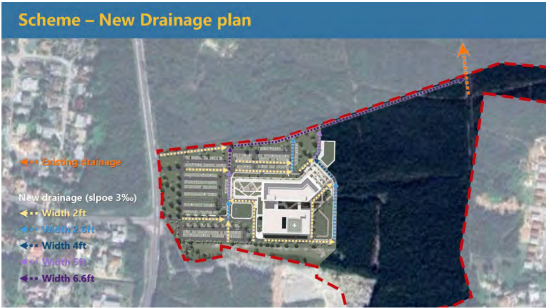
Figure 19: New drainage at The Project site
