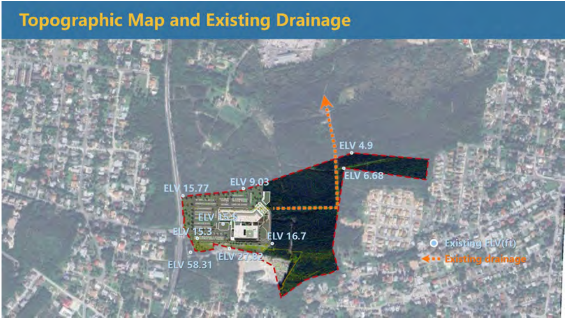
Figure 18: Existing drainage at The Project site
