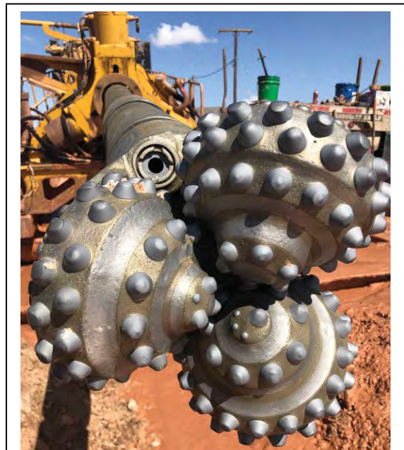
Typical downhole hydraulic motor with rock bit for cutting hard rock
