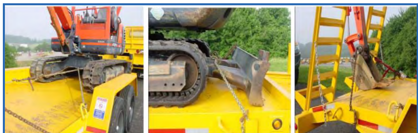
Figure 9g Excavator Securement
