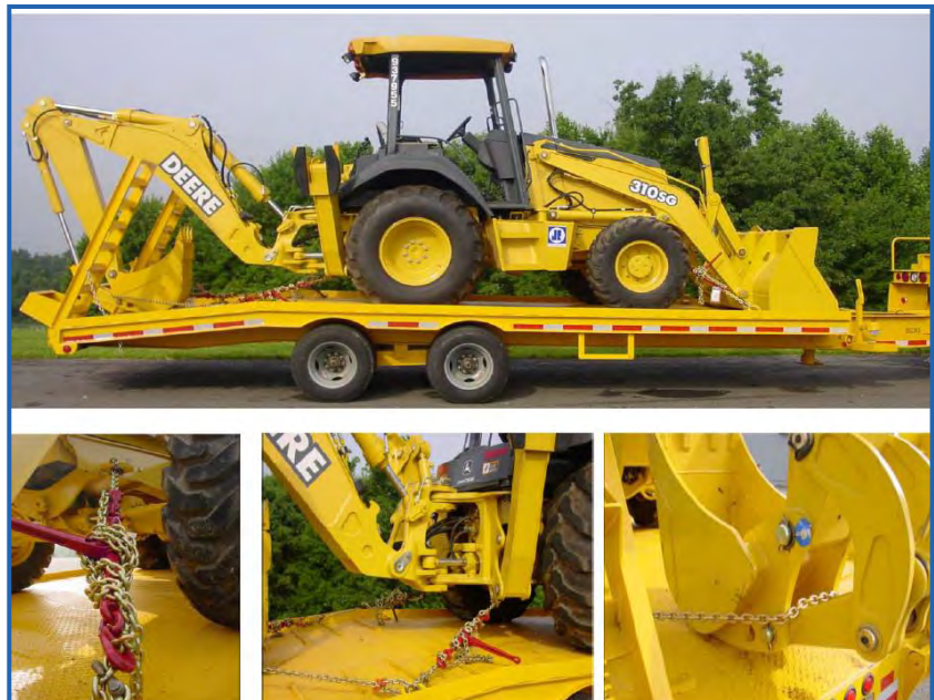
Figure 9f Securement of Heavy Equipment
