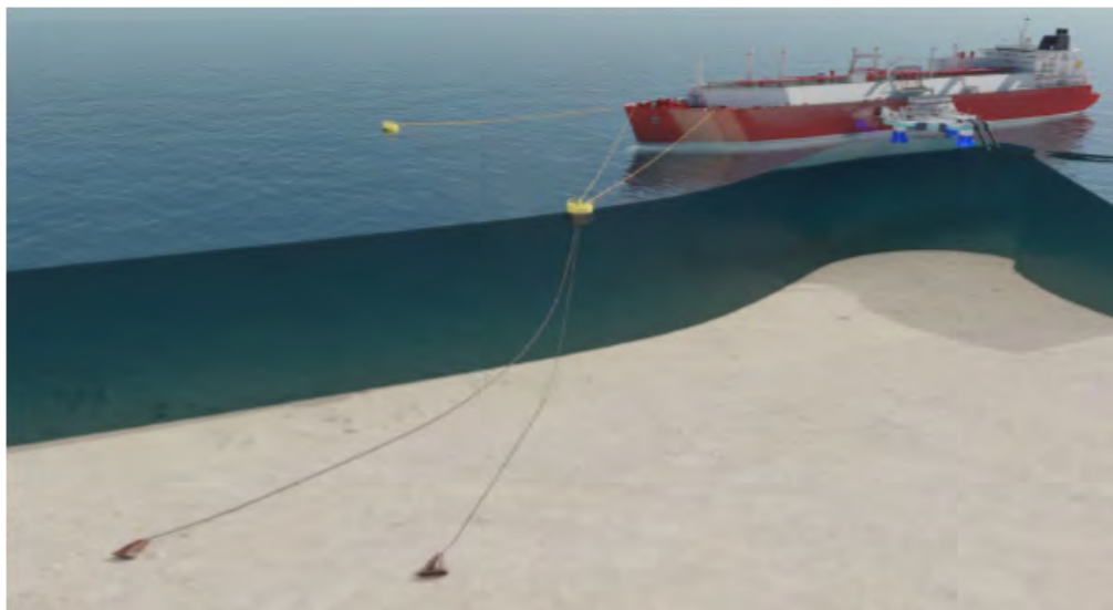
Figure 4: Conventional Buoy Mooring System (CBM) or Multi Buoy Mooring System (MBM)
